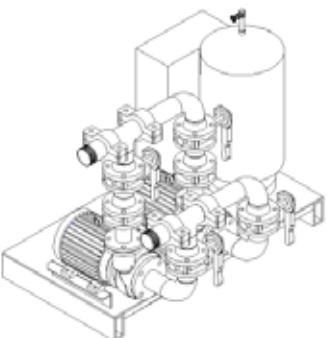
Total System Head \_\_\_\_\_ ft-H<sub>2</sub>O = Highest Fluid Cooler Pressure Drop \_\_\_\_\_ ft-H<sub>2</sub>O + Highest Evaporator Unit Heat Exchanger Pressure Drop (i.e. Cond. As per below in Chiller) \_\_\_\_\_ ft H<sub>2</sub>O + Pressure Drop of Supply & Return Glycol Piping + All Valves & Fittings \_\_\_\_\_ ft-H<sub>2</sub>O
