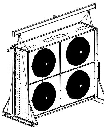
Ensure the unit is placed in a level position (to ensure proper drainage of fluid). The legs should be securely anchored to the building structure, sleeper or concrete pad. The weight of the fluid cooler alone is not enough to hold in place during a strong wind, the legs must be anchored.
